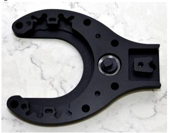
m) Install the selector knob snap ring into the groove on selector knob. This will require slightly depressing the wave spring.
