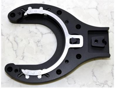
c) Carefully spread one pair of pawls and insert the center pin on that side of the selector into the slot between the pawls. Both outer pins on the selector should be inside each of the pawls.
