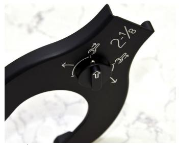
h) Carefully compress the 1/8<sup>th</sup> inch bearing ball and spring into the selector knob using the end of a small flat bladed screwdriver. Take care to avoid releasing the spring and launching the bearing ball.
